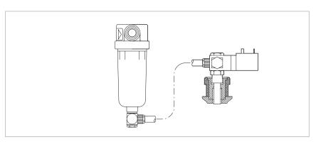
AR-V oil suction facility controlled by solenoid valve (kit without exhaust filter)
