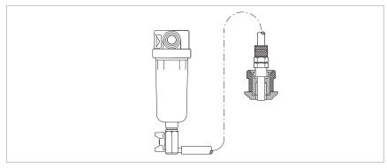
AR-M manually operated oil suction facility (kit without exhaust filter)
