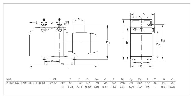
Dimensional drawing for the TRIVAC D 16 B-DOT
