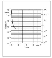
Pump-down characteristics of a 10 I vessel at 50 Hz
