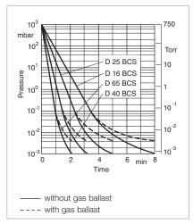
Pump-down characteristics of a 100 I vessel at 50 Hz
