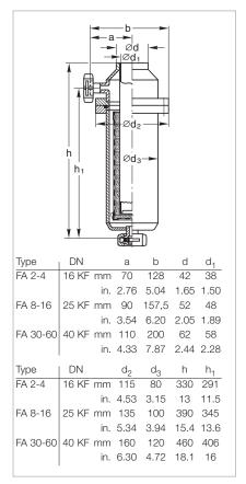
Dimensional drawing for the FA fine vacuum adsorption trap
