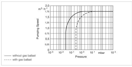
Pumping speed characteristics at 50 Hz
