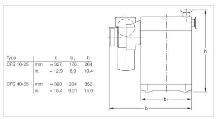
Dimensional drawing for the CFS (mounted on a TRIVAC BCS)
