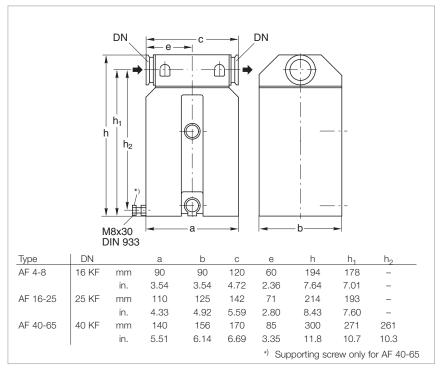
Dimensional drawing for the AF exhaust filter
