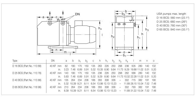
Dimensional drawing for the TRIVAC D 16 to D 65 BCS
