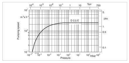
Pumping speed of the TRIVAC D 2,5 E at 50 Hz (60 Hz curves at the end of the section)
