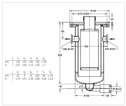
Dimensional drawing for the TK 4-8 cold trap
