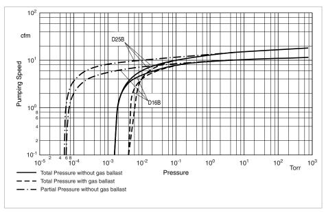
Pumping speed characteristics for the TRIVAC D 16 B/BCS and D 25 B/BCS at 60 Hz
