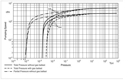
Pumping speed characteristics for the TRIVAC D 4 B and D 8 B at 60 Hz
