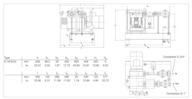
Dimensional drawing for the TRIVAC 16 B-Ex (explosion protected and pressure burst resistant)
