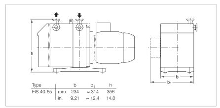
Dimensional drawing for the EIS (mounted on a TRIVAC BCS)
