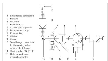
Example of connecting a pump with accessories
