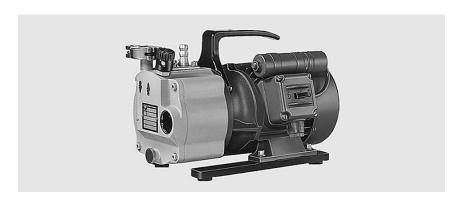
The S 1,5 is a single-stage, oil-sealed rotary vane pump with a gas ballast valve. It is driven by a flange mounted AC motor. The shaft of the pump and the shaft of the motor are linked by means of a pinned coupling.
