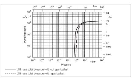
Pumping speed characteristics at 50 Hz (60 Hz curves at the end of the section)
