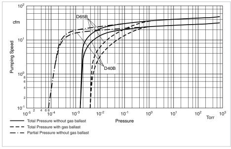
Pumping speed characteristics for the TRIVAC D 40 B/BCS and D 65 B/BCS at 60 Hz
