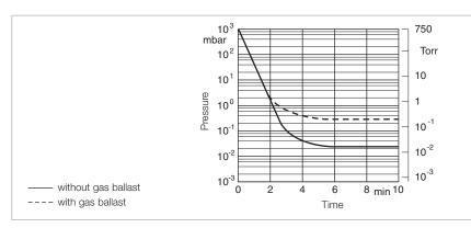
Pump-down characteristics of a 10 I vessel at 50 Hz
