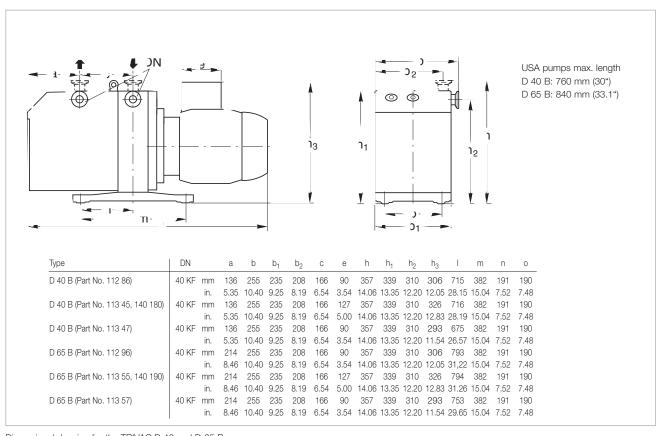
Dimensional drawing for the TRIVAC D 40 and D 65 B
