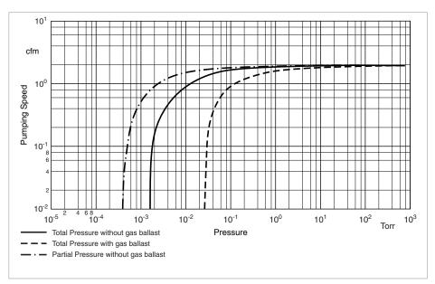
Pumping speed characteristics for the TRIVAC D 2.5 E at 60 Hz
