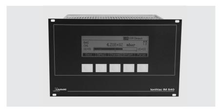
The 3-channel display and operating unit IONIVAC IM 540 offers, by combination of up to 4 different principles of measurement – Pirani, capacitive, Bayard-Alpert and Extractor–, complete coverage and control of the vacuum pressure in the range between 10<sup>-12</sup> mbar and atmospheric pressure.
