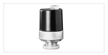
The PENNINGVAC transmitter combines the cold cathode ionization principle with the Pirani principle. This allows for complete coverage of the pressure range from 5 x 10<sup>-9</sup> mbar to atmospheric pressure by a single transmitter. The cold cathode system is ignited directly through switching on the internal high-voltage at the optimum ignition pressure.
