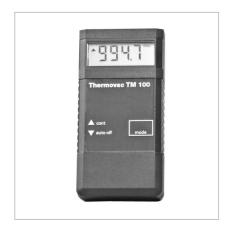
The handheld THERMOVAC TM 100 is capable of measuring pressures within the pressure range of 5 x 10<sup>-4</sup> to 1200 mbar. By combining a piezoresistive pressure sensor for the upper and a Pirani sensor for the lower pressure range, the measurements made by the THERMOVAC TM 100 are independent of the type of gas above pressures of 15 mbar. Especially noteworthy is the exceptionally long battery life.
