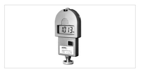
The THERMOVAC TM 90 is a simple handheld vacuum measuring instrument for occasional use. Its operation is based on the Pirani principle and covers a measurement range from 1 x 10<sup>-2</sup> mbar to atmospheric pressure. It is delivered in a rugged plastic
