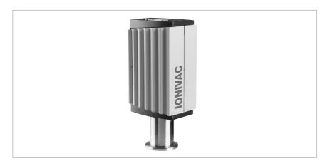
The ITR 200 S is an optimised dual cathode combination transmitter on the basis of the well proven ITR 90. The combination of a hot cathode ionization sensor according to Bayard-Alpert and a Pirani sensor allows vacuum pressure measurements of non-ignitable gases and gas mixtures in the pressure range from 5 x 10<sup>-10</sup> to 1000 mbar.
