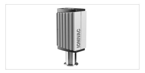
The ITR 90 is a optimized combination transmitter. The combination of a hot cathode ionisation sensor according to Bayard-Alpert and a Pirani sensor permits vacuum pressure measurements of nonignitable gases and gas mixtures in the pressure range from  $5 \times 10^{-10}$  to
