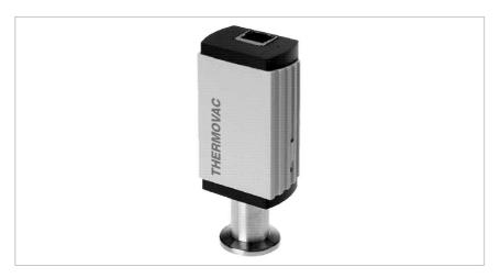
The Pirani Capacitance Diaphragm Gauge is the first vacuum gauge which combines ceramic capacitance diaphragm and thermal conductivity technologies. Unlike standard heat transfer technology, the Oerlikon Leybold Vacuum TTR 100 offers superior accuracy and gas-type-independent readings between 100 mbar and 1500 mbar.
