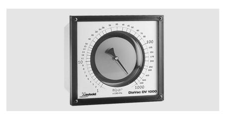
Rugged mechanical diaphragm vacuum gauge of high accuracy for the rough vacuum range from 1 to 1000 mbar (1 to 750 Torr).
