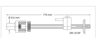
Calibrated leak with pin type casing and VCO fitting
