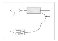
Leak detection -Search gas overpressure in the test object
