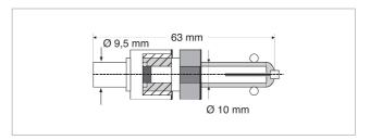
Calibrated leak with cylindrical casing and VCO fitting
