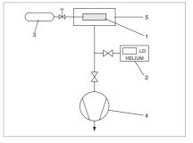
Integral methode -Search gas overpressure in the test object
