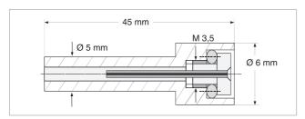
Calibrated leak with screw-in sleeve
