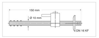
Calibrated leak with pin type casing and hose nozzle
