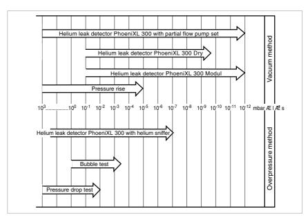
Overview of the leak rate detection ranges
